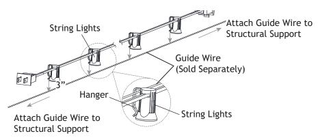
Pass the guide wire through the holes on the top end of the sockets and then fix the guide wire to your desired location or tie the bistro string to applicable locations directly.
