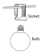
Tighten the UL Classified bulbs (5 watt Max Candelabra-base) into the socket clockwise until the top of the socket forms a tight seal around the bulb and the bulb makes solid contact with the socket.
